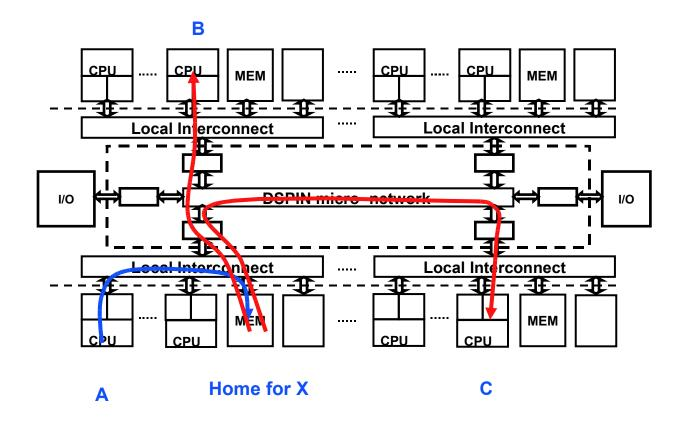
CPU A makes a write to an address X CPUs B & C have a copy
