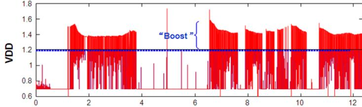
In a DRM System, the maximum voltage can be "boosted" to allow periods of higher peak performance while maintaining a margin below the budgeted damage curve.
