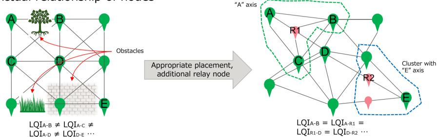
Even though the physical distance is symmetric, it will not be symmetric in terms of wireless communication
