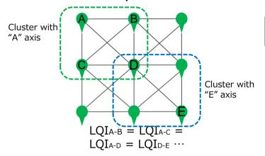
Data calibration operation with neighbor nodes Reliable data transfer (ad-hoc network)
